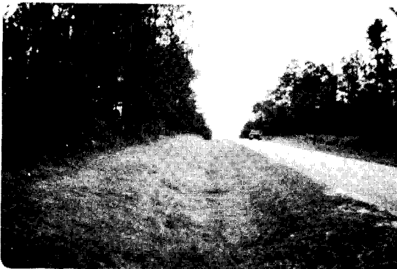
Figure B-4 Test Channel No. 1-FGR with permanent grass liner established with aid of fiber glass roving.
